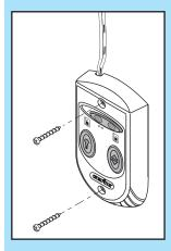
FIG. 3-4 Mounting Wall Console.
